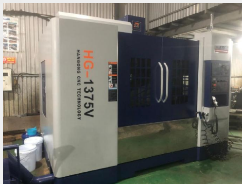
Vertical high speed machining center X axis: 1300mm ; Y axis: 750mm; Z axis: 600mm Positioning accuracy: 0.01mm; Rotation speed : 8000rpm
